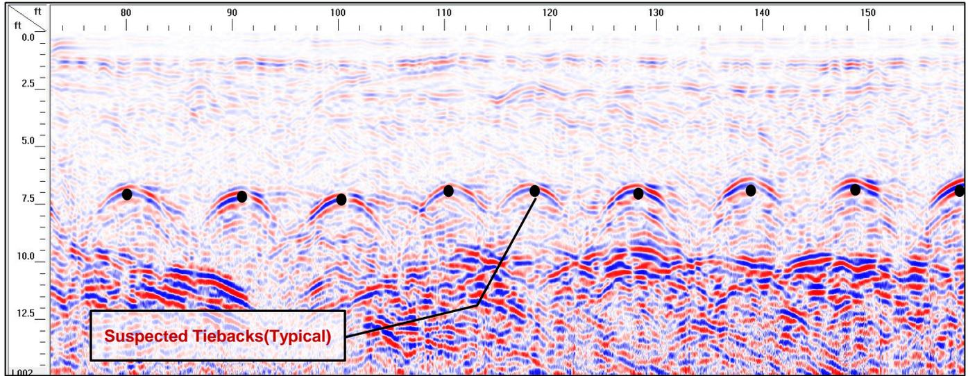
**Transect T-6** - Example GPR profile approximately 25 feet west of the seawall (north to south direction). Tiebacks spaced approximately 10 feet on-center. The depth shown is approximate.
